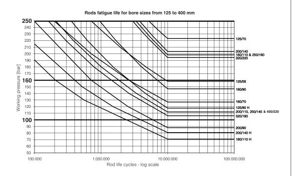
**Note:** the curves are labelled according to the bore/rod size. The light male thread (option  $\mathbf{H}$ ) is indicated by the "H" after the rod Example: label **125/90 H** means bore = 125 mm, rod = 90 mm and rod with option  $\mathbf{H}$
